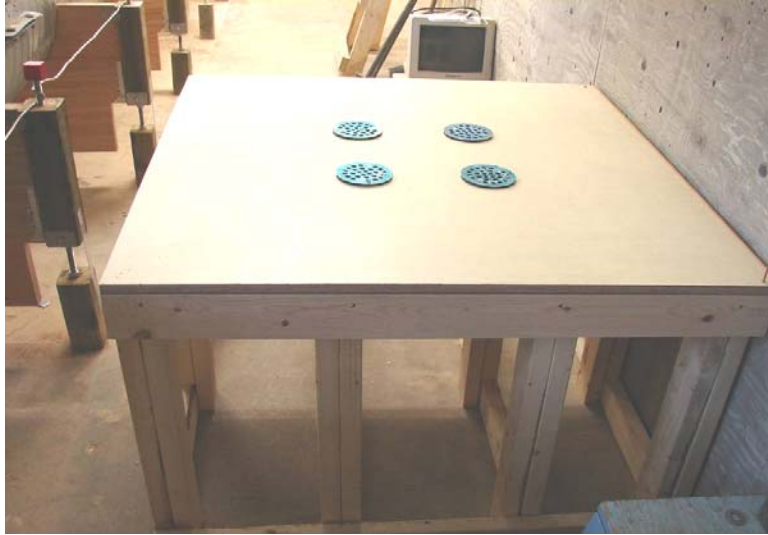
Figure 2. Elevated floor of the setup
