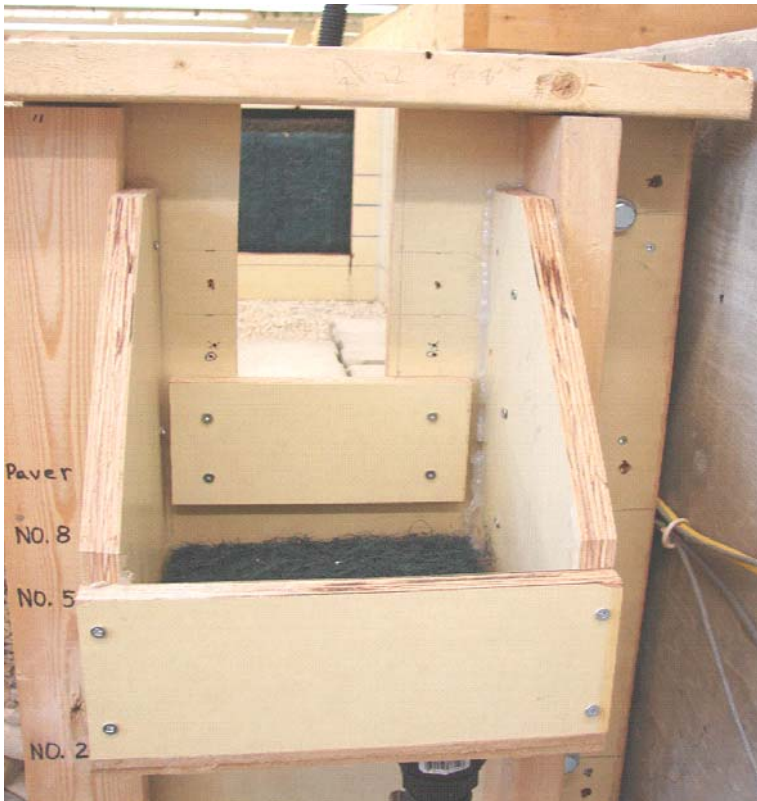
Figure 5. Overflow to ensure constant head of water
