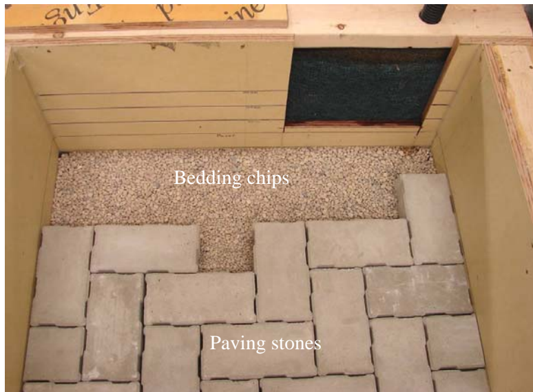
Figure 7. Herringbone paving block pattern
