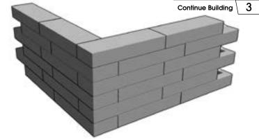
Repeat until desired wall height is achieved. Finish the corner off with a closed-end coping block.
