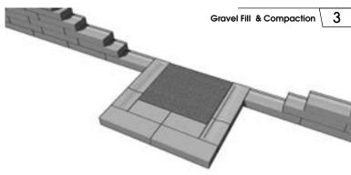
Fill the reinforced zone with imported, free draining gravel and compact to 95% SPD.
