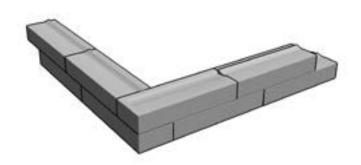
Commence second course by flipping a corner block and placing it in the alternate direction. Place standard blocks to complete the course.
