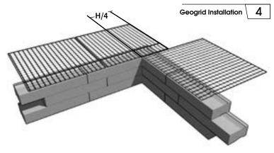
The geogrid should be placed within 1"(2.5cm) of the face of the block. As it is only necessary to have geogrid extending directly away from the wall, a gap will result in the geogrid layer as shown.
