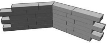
Repeat until desired wall height is achieved. Finish off with two cut coping units. The angle of the cut for the coping blocks should be half the angle of the final wall corner (eg. 22.5° for a 45° corner).
