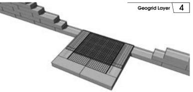
course of steps reduces the effect of settlement. It is recommended to include an additional geogrid layer every other step placed in the perpendicular principle direction.
