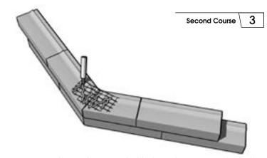
Commence second course by cutting the blocks on the opposite side so when installed, it will create an overlapping bond pattern as shown. Place the cut blocks in the corner and use standard blocks to complete the course.
