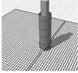
To place the sonotubes, cut the geogrid perpendicular to the wall along the centerline of the sonotube, creating two geogrid panels - one on each side of the sonotube. Lay the geogrid flat in front of the sonotube. At the intersection with the sonotube, fold the geogrid flat against vertical side of the sonotube and then around the back, maintaining the edge of the geogrid along the centerline of the sonotube. Lay the geogrid flat behind the sonotube and pull taut.
