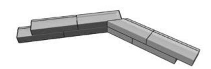
Commence second course by cutting the block on the opposite side so when installed, this will create an overlapping bond pattern as shown. Flip and place a corner block in the alternate direction. Place the cut block in the corner and use standard blocks to complete the course.
