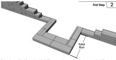
Start the wall with two inside 90° corners (page 9) and two outside 90° corners (page 8) using closed-end coping blocks. Use the Total Run formula to determine the distance out from the face of the wall where the front of the first riser should be placed. Place another row of coping blocks back-to-back directly behind the first set.
