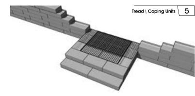
Place the next course back to the desired tread depth. For best results offset the cuts to create a bond pattern with the step below. Fill the reinforced zone with imported, free draining gravel and compact to 95% SPD. Place a geogrid reinforcement layer.
