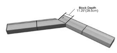
Place blocks on the base course leading to the corner. Place the cut block and align a corner block as shown, insetting corner block a minimum of 11.25" (28.5cm) (Block Depth) from the edge. Place standard blocks to complete the course.
