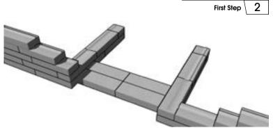
Start the wall with two outside 90° corners (page 8) distanced as specified in the Design. Place coping blocks between to form the first step riser, measure and cut if required. Place another row of coping blocks back-to-back directly behind the first set.
