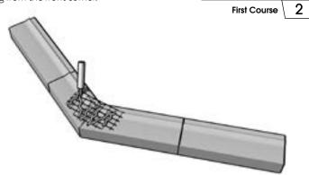
Place blocks on the base course leading to the corner and use the cut corner blocks. Place standard blocks to complete the course.
