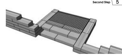
Place the next course back to the desired tread depth. For best results offset the cuts to create a bond pattern with the step below. Fill the reinforced zone with imported, free draining gravel and compact to 95% SPD. Place a geogrid reinforcement layer.
