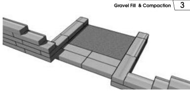
Fill the reinforced zone with imported, free draining gravel and compact to 95% SPD.
