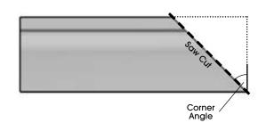
Using one standard block prepare and cut the blocks as shown. The angle of the cut should be the same angle as the final wall corner. Cut the block starting from the front corner.
