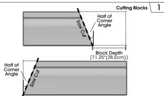
Using two standard blocks, prepare and cut the blocks as shown. Mark the first block insetting the cut line 11.25"(28.5cm) (Block Depth) from the front edge. The angle of the cut should be half the angle of the final wall corner (eg. 22.5° for a 45° corner). Cut the second block at the same angle on the oposite side starting from the front corner.
