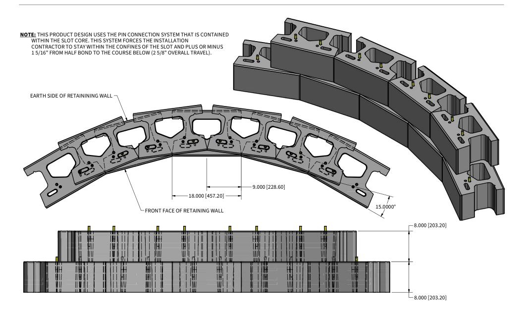
Retaining Exterior Radius/Curved Wall Installation Shown In Near Setback Pin Position
