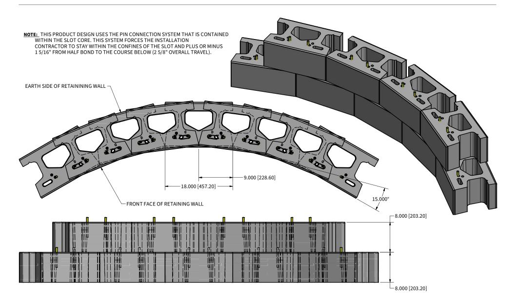
Retaining Interior Radius/Curved Wall Installation Shown in Full Setback Position
