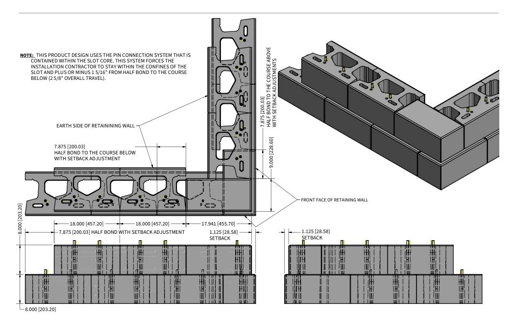
Retaining Exterior 90° Corner Wall Installation Shown in Near Setback Pin Position
